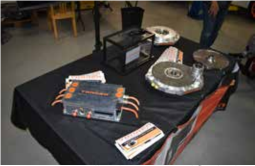
Vonnen Controller, drive motor and flywheel
