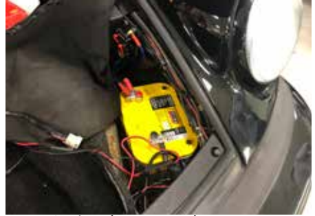
Optima battery replacement
